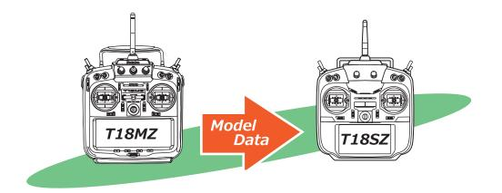
The T18SZ Model Data Converter is software that converts model data for T18MZ to that for T18SZ. The software cannot convert model data made by other transmitters such as T14MZ etc. Thus please still use the existing converter - Futaba Model Data Converter Ver.1.0.4, if you want to convert model data for T14MZ/FX-40/T12Z/T12FG/FX-30.
