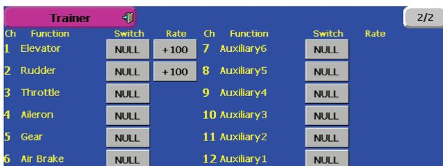
Set the trainer mode to either MIX or FUNC mode. The rate buttons appear on the 2nd page of the trainer screen. Set the student rate as desired.
