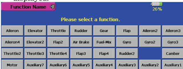
3. Select the function to be renamed and press the [Rename] button. A character input screen is displayed. Type in the new function name and press [Enter] to store the new function name, or press [Esc] to cancel.
