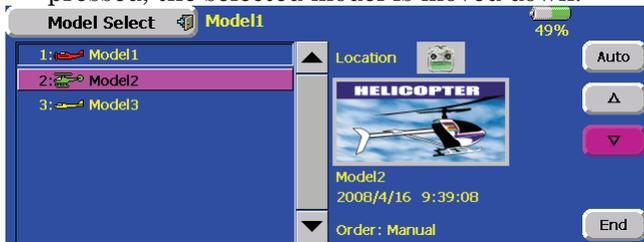
3. When the [Auto] button is pressed, the [Name] and [Date] button is displayed. When the [Date] button is pressed, the display is switched to the date order mode, and when the [Name] button is pressed, the display is switched to the name order mode.
