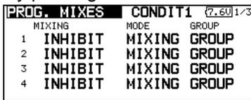
2. Use [MODE] setting to select the program mixing operation mode. [MIXING] is the normal mixing mode and [OFFSET] is the offset mode.
