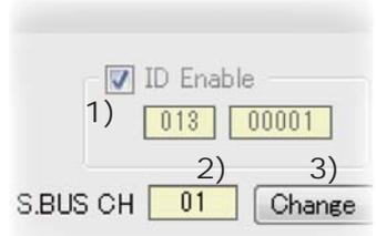
When connecting multiple servos to the CIU-2/3 tick the "ID Enable" check box, input the ID No. of the ID seal attached to the servo whose parameters are to be read, and click the "Connect" button or select "Connect" from the "Tool" menu. If the ID is a mismatch, the Error message shown below (right side) will be displayed and communication will not be established.
