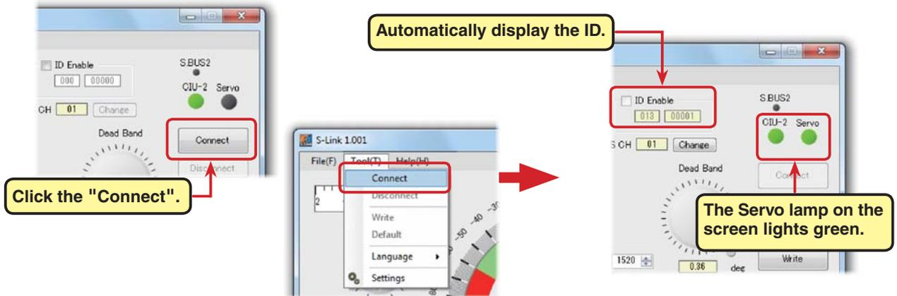
When connecting multiple servos simultaneously using a S.BUS hub tick the check box at the left side of "ID Enable", input the ID of the servo you want to set, and click the "Connect" button. The current setup parameters of that servo are displayed and the Servo lamp on the screen lights green.
