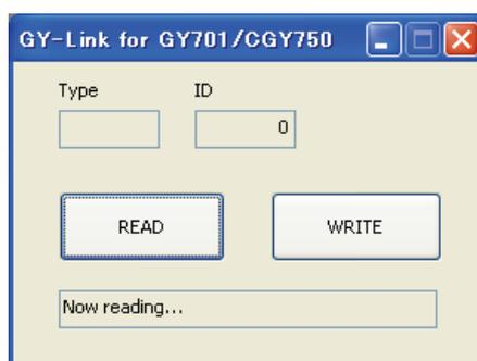
5). When complete the reading, the box shows model type and ID number. When you have Read error message or box does not show the ID number, make sure the wire connection and power supply and retry the reading process again.
