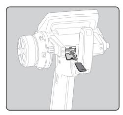
6. Turn on the transmitter power while pressing down the "END" button. The update screen appears on the LCD display of your T4PX and the software update is started.
