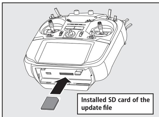
6. Turn on the transmitter power while pressing down the "HOME/EXIT" button. The update screen appears on the LCD display of your T18SZ and the software update is started.
