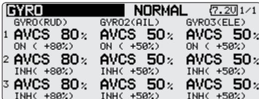
2) When a gyro function button is chosen, the detailed setting screen of each gyro is displayed.
