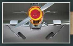
Mechanical retracts made of high quality composite allow for even more in-flight realism.
