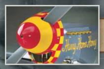
An aluminum spinner and molded dummy exhaust pipes add to the authenticity.
