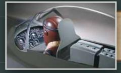
Under the vacu-formed canopy is a detailed cockpit including instrument panel, seat back rest and dummy radio boxes.
