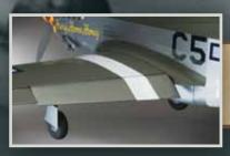
Flaps are already built into the Mustang ARF's wings; modelers simply add servos.
