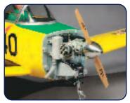
The Mentor will fly well with a .61-size 2-stroke engine like the one shown here; a 4-stroke power plant will also fit inside the cowl.
