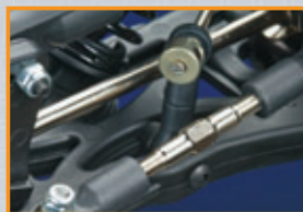
Optimized servo positioning lowers the CG and turns the arm and linkage inboard to eliminate impact damage.
