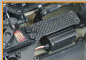
Optimized servo positioning lowers the CG and turns the arm and linkage inboard to eliminate impact damage.
