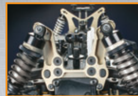
Hard anodizing and CNC-machining helps the Z01-B's lightened aluminum towers outlast anything the track dishes out.
