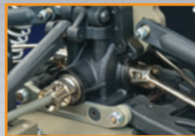
Outdrives are machined, lightened and nickel-plated, to reduce weight and wear.
