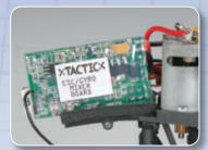
The electronics responsible for controlling speed and keeping the AXE EZ level are dependable, protected - and preinstalled.
