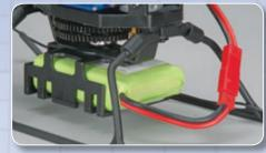
Positioned for in-flight stability and easy access, the 800mAh LiPo battery pack is good for 10-15 minutes of flight per charge.
