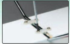
The wire landing gear simply plugs into the bottom of the Hobbistar MKIII's fuselage. It's held in place by landing gear straps which fasten into predrilled holes.
