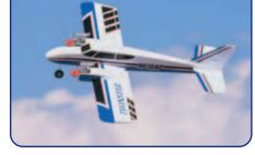
Even with its dual engines, the TwinStar handles much like a single-engine R/C plane of comparable size. Careful positioning of the centerline ensures that the TwinStar is still flyable even if one of the engines stops!
