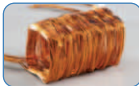
Each winding starts out as a hollow rectangle of fine copper wire...
