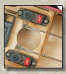
Quality ElectriFly micro servos are included and installed in the Rx-R version and ready to be hooked up to the receiver.
