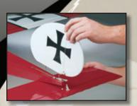
No gluing or measuring! The horizontal and vertical stabs simply bolt together.
