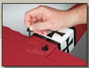
The wing attaches quickly with these two streamlined thumb screws — no tools required!
