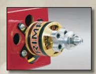
A powerful RimFire 42-40-1000 out-runner brushless motor is already in place on the ElectroStik Rx-R, and is easy to mount in the ARF version.
