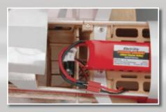
Magnetic latches on the cowl and battery hatch eliminate the need for screw fasteners — producing cleaner looks and improving aerodynamics. The magnets hold firmly in place during flight, but release quickly and easily for motor checks and LiPo pack changes.
