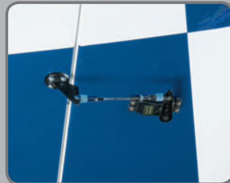
Each aileron is controlled by an individual servo. Short, direct linkages make roll control precise, positive, dependable and easy to set up.
