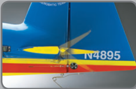
Large control surfaces and full deflection throws enable the Edge 540 to react quickly to 3D control inputs. The rudder and each elevator half utilize independent servos for consistent yaw and pitch control. Servos can be mounted in the fuselage for a lightweight pull-pull setup, or in the tail for a shorter, more direct linkage.
