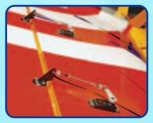
Each wing half of the 1/3 scale Matt Chapman CAP 580 uses two servos to actuate its aileron control surface. This provides the muscle for crisp deflection, enabling the model to excel in 3D aerobatics and IMAC competition as well as during "everyday" sport flying.
