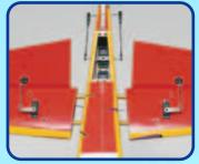
Like its main wing, the CAP 580's stabilizer halves slide onto aluminum joiners and remove easily for transport. Each half has its own servo for elevator actuation. The steerable tailwheel provides positive ground handling.
