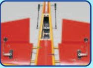
Stabilizer halves, each with its own elevator servo, slide onto aluminum joiners and remove easily for transport. Positive rudder control is provided by dual servos, which are coupled using supplied linkage hardware created expressly for large-scale models.
