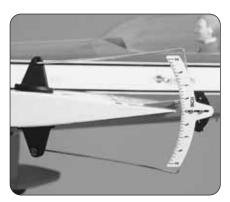
Accurate control throws add predictability to performance and reduce the chances of damage due to too little-or too much-control. With the AccuThrow, you can check control throws before you fly. It's incredibly easy to use-rubber feet provide a firm grip, while spring tension holds the ruler (curved to match control motions) steady. **GPMR2405**
