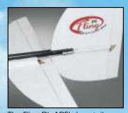
The Fling DL ARF's long tail contributes to aerodynamics that result in powerful discusstyle launches. Rudder and elevator control surfaces are actuated using a lightweight, easy-to-install pull/pull linkage system.
