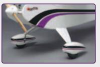
Stylish covers encase the wire landing gear to enhance the plane's looks. The ABS wheel pants speed assembly by eliminating tedious shaping work.
