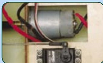
An ESC, 550 motor and direct-drive system combine for smooth, powerful maneuvering in forward and reverse.
