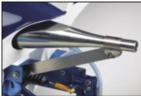
The engine's tuned pipe is made of spun aluminum, and comes with a stainless steel support bracket and exhaust header with gas coupler.
