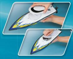
Easy-access, waterproof compartments in the durable, lightweight ABS hull protect the on-board electronics.
