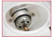
Includes a powerful, water-cooled 380-size electric motor for high speed action.
