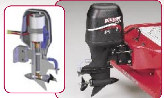
From the shaft down, the EP outboard is all cast-aluminum and stainless steel. Other features include a water-cooled 550 motor, ball-bearing drivetrain and an adjustable transom mount. EP outboard also sold separately (HCAB7861.)
