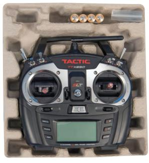
Your Tactic TTX650 six-channel radio comes with four "AA" batteries for power. You can change them out for either NiCads or NiMH cells.
