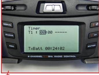
The timer gives you 99 minutes and 59 seconds of count time. As you would expect, the timer can be controlled by any switch or control function.
