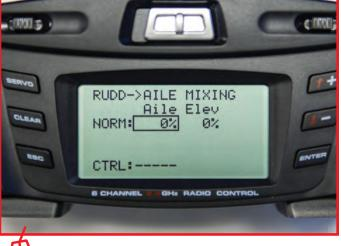
As you can see you set the amount of aileron to rudder mixing that you want for your model. You can also select the switch that can turn the mixing on and off.
