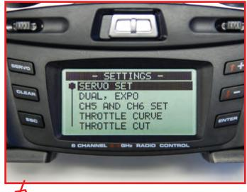
These are the additional programming functions that are available under the Settings menu. You'll move up and down in the menus using the up and down arrow keys.
