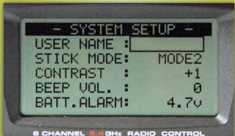
The system setup menu is where you can set overall system options for the transmitter.
