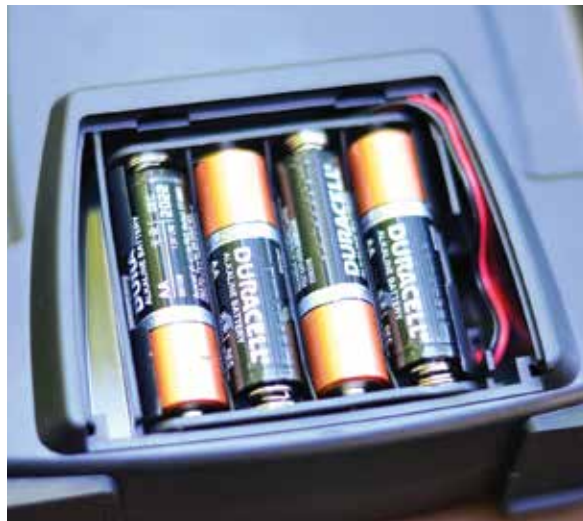
The radio uses four AA batteries, with the option of adding a rechargeable pack.
