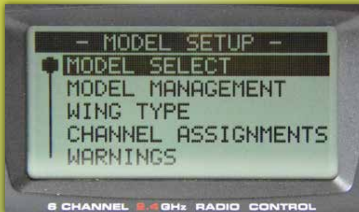
The model setup menu is where you can manage models and set wing types and channel assignments.
