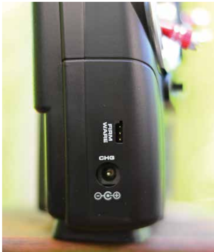
The charge jack for the optional rechargeable battery and the firmware update port requires an additional cable.
