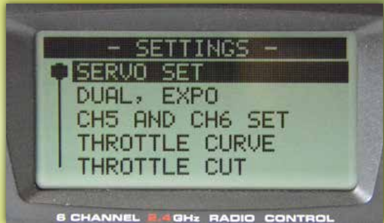
The settings menu shows some of the available servo setup options.
