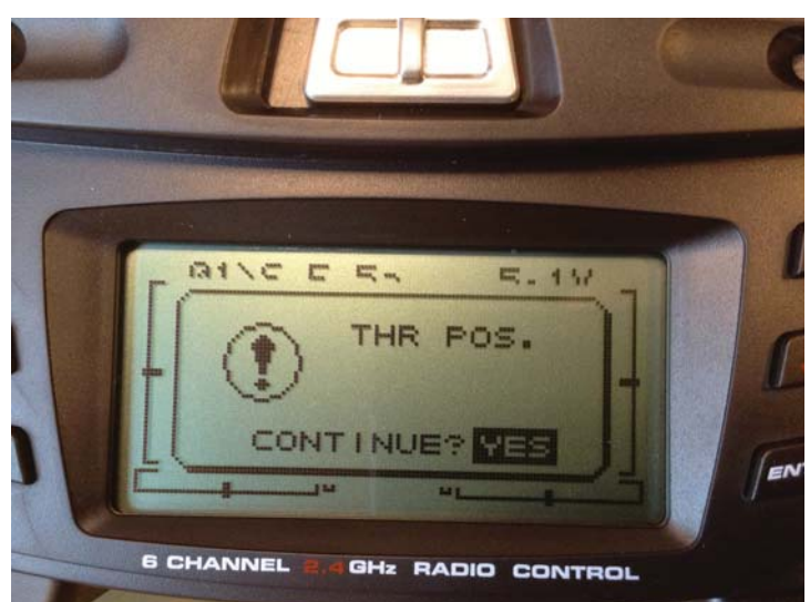
(below left); however, these can be replaced by a rechargeable Ni-MH pack. Text has details. Should you leave the throttle position at anywhere but bottom, the TTX650 will force you (below right) to either lower the throttle position or select the ENTER key to continue.
