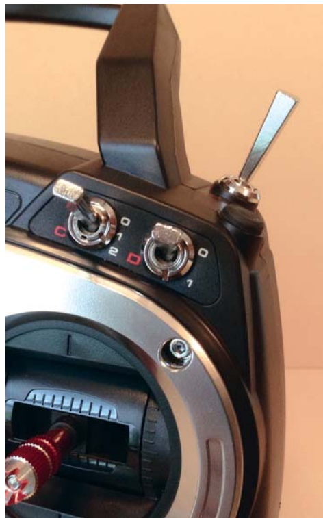
The Tactic TTX650 may be an economical sport radio, but don't let its price fool you, it's loaded with features. The ergonomic case (above left) is sculpted for many hours of comfortable flying. Two and three position switches (above right) are selectable through easy programming for programmable mixes and dual rates.
