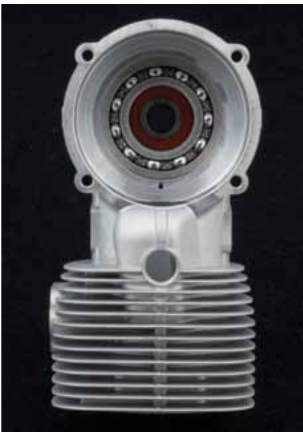
↗ O.S. uses a one-piece casting for the crankcase and cylinder. Note how large the rear ball bearing is, allowing almost a full view of the front bearing, which uses rubber seals. Also note the hole through the casting wall in the rear transfer port—this allows access to remove and install the piston pin.
