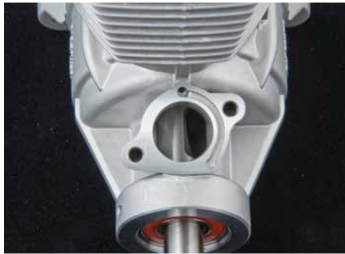
With the carburetor and plastic spacer removed, you can see the rotary-valve intake passage in the crankshaft (positioned to show the port half-way open in this photo). The small hole above the intake port goes through to inside of the crankcase, and the curved slot in the casting allows the crankcase pressure pulse signal to reach the carburetor to drive the fuel pump diaphragm.
