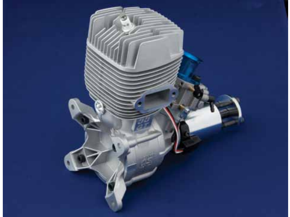
⤴ This right rear view shows how heavily finned the cylinder and head are, which makes for excellent cooling, and also the lightweight but rigid backplate, which serves as the engine mount.
