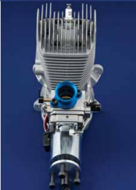
⤴ This right rear view shows how heavily finned the cylinder and head are, which makes for excellent cooling, and also the lightweight but rigid backplate, which serves as the engine mount.
