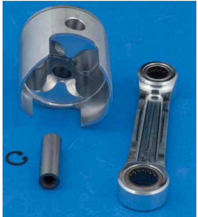
↗ Here you see the results of some fine CNC machine work at the O.S. factory. The piston and connecting rod are CNC-machine made from bar stock, and the connecting rod is fitted with needle roller bearings at both ends. The piston pin is retained by a pair of C-clips. These are quality made parts, which result in an engine that performs well.
