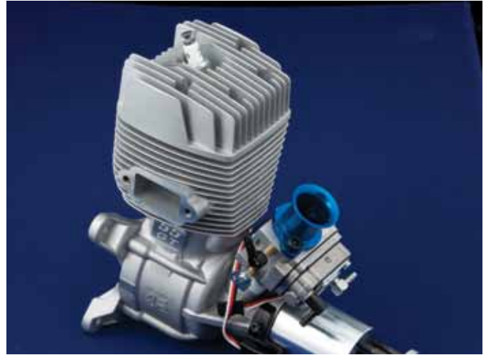
⤴ The rather large exhaust port is on the right side of the engine, as is the ignition sensor. The right side of the carburetor has the fuel inlet fitting and the choke lever. The spark plug slants to the rear as well.
