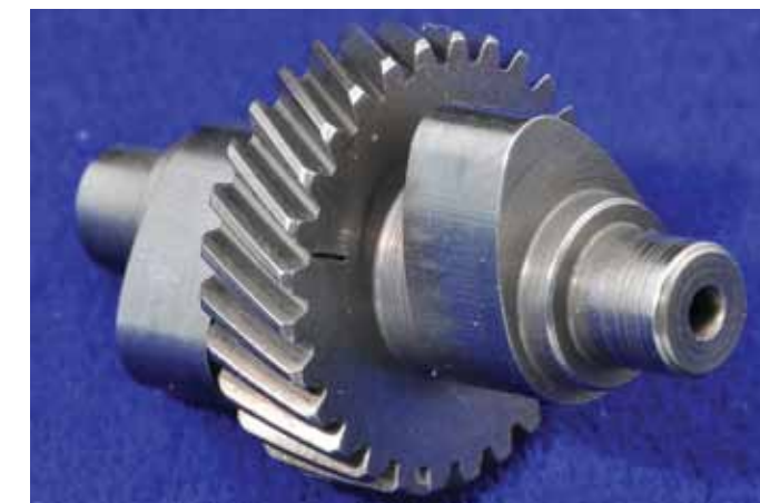
▶ Here is a close-up of the crankshaft, showing the helical-cut gear teeth, lobes, and alignment mark used to assure correct timing during installation.
