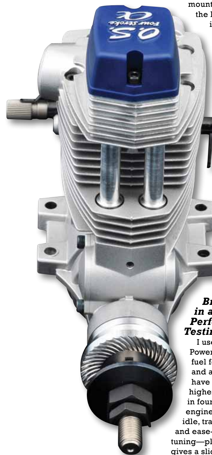
↗ This front view clearly shows the new cooling fin arrangement, narrow profile, and machined-aluminum pushrod tubes. The new logo on the rocker cover is also a nice touch!
