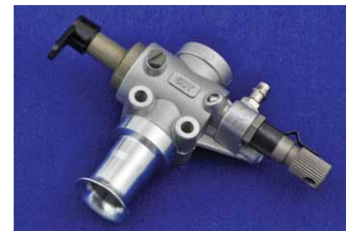
▶ The 60Y carburetor is reversible and has proven to perform well and tune easily. The extended venturi tube helps minimize reversion (spit-back of fuel out of the carb inlet) which makes the engine cleaner-running and a bit more fuel efficient.
