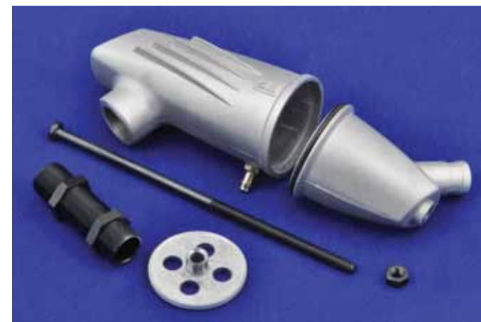
▶ The F-5040 muffler allows substantial installation flexibility since the muffler can be rotated a full 360-degrees; the outlet can be angled by rotating the rear muffler part relative to the front.
