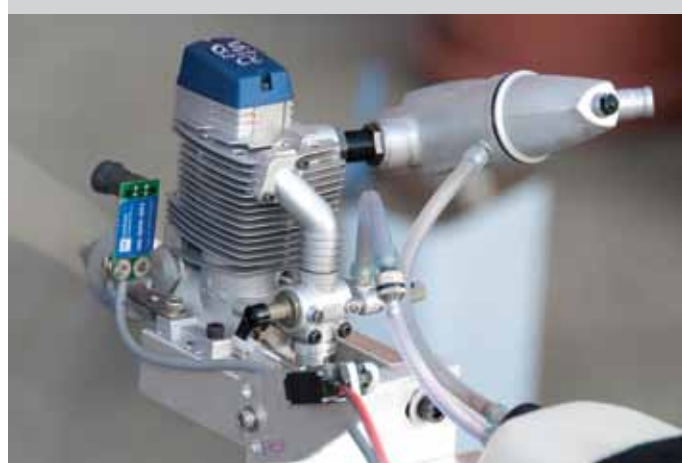
The 110FS-a is attached to the test stand via adjustable mount legs. The small circuit board just behind the propeller hub is the optical tachometer, which is part of the Medusa Research "Power Analyzer Pro" data system.
