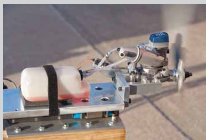
The 110FS-a is attached to the test stand via adjustable mount legs. The small circuit board just behind the propeller hub is the optical tachometer, which is part of the Medusa Research "Power Analyzer Pro" data system.
