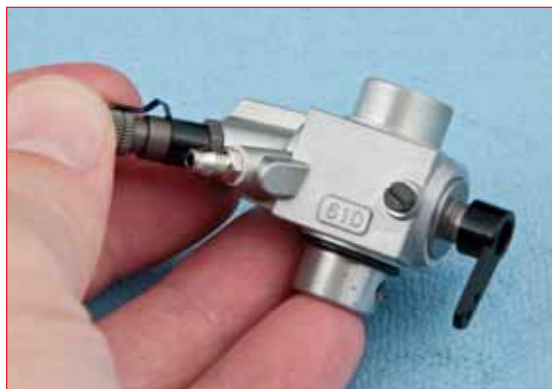
The 61D carburetor works great, plus offers a new 45-degree orientation of the high-speed needle valve. This keeps your fingers well clear of the propeller, while eliminating the need for a remote needle valve.
