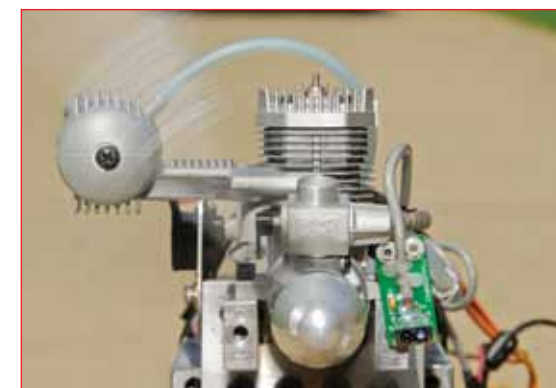
This gives you a close-up view of the O.S. 65AX in action! The small green circuit board is the optical tachometer pickup that provides a signal to the Medusa Power Analyzer Pro box.
