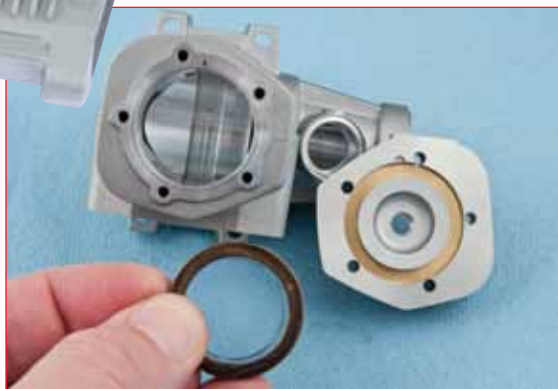
This view of the main cylinder casting, the cylinder sleeve, and the cylinder head show how the small roll pin is used to assure perfect alignment of the cylinder, and therefore the transfer and exhaust ports.
