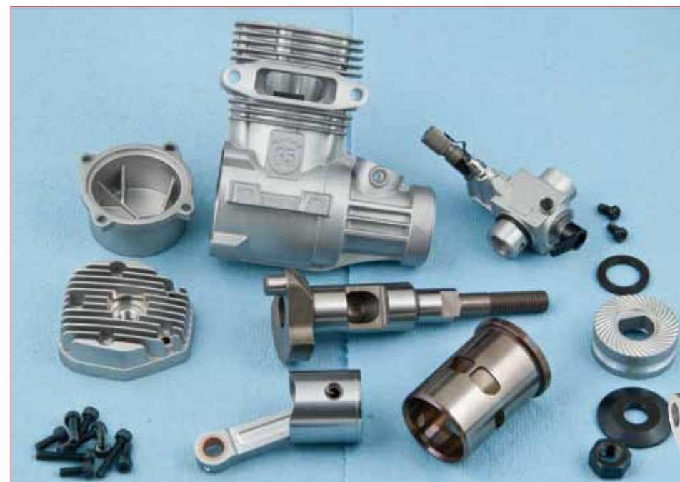
This is a layout of the 65AX parts. Use of o-rings, rubber seals, and a metal head shim make teardown and re-assembly a snap. Note the sturdy connecting rod with bronze bushing, and long-skirt piston design.
