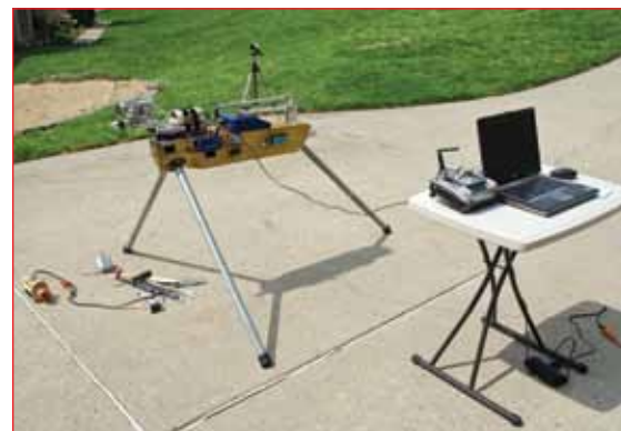
Here you see the overall test stand and equipment arrangement. A sound level meter is mounted to a camera tripod (in the background), and the PC that controls and monitors the thrust test stand is to the right, on a small folding table.
