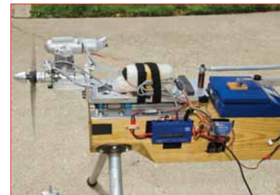
The O.S. 65AX is running on the thrust test stand, with a Master Airscrew 13x5 composite propeller attached. The throttle servo is commanded via PC control for a test run, with all data being displayed and recorded by the computer via the Medusa Power Analyzer Pro data system.
