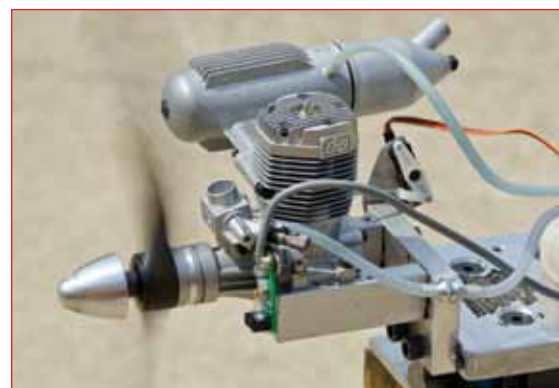
This gives you a close-up view of the O.S. 65AX in action! The small green circuit board is the optical tachometer pickup that provides a signal to the Medusa Power Analyzer Pro box.
