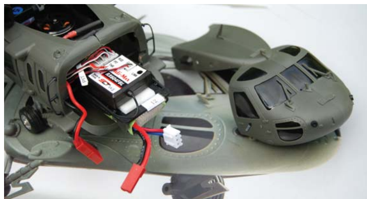
Battery access on the Black Hawk is gained by the removable nose (above), which is held in place with magnets. Care must be taken when removing and re-installing it due to the small antennas flanking it. The real thing about to make a troop drop or micro R/C model (at right)? With all that incredible detail sometimes it's tough to tell!
