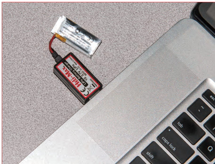
Charging the 1S 250-mAh LiPo battery is as easy as plugging the charger into a computer, cell phone, or other USB port. The charger charges at the rate of one C.
