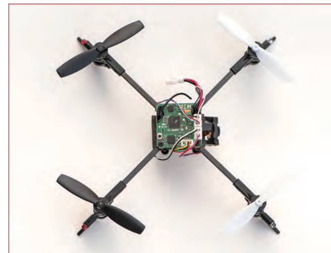
This photo gives you a good look at what the guts of the Heli-Max ISQ V•CAM look like. There is lots and lots of "brain power" packed into the microprocessor on this quad.
