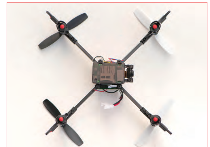
Here you can see where the SD card plugs into the bottom of the quad, as well as the camera. The battery holder sits just above the camera mount and the battery slides in from the back.
