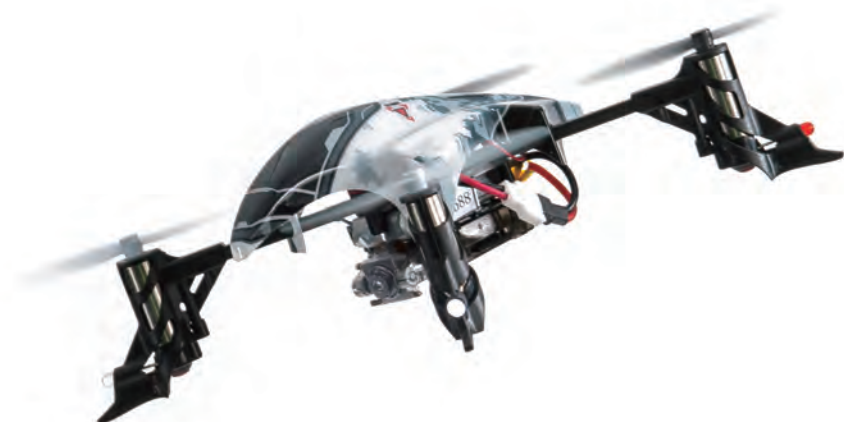
As you can see, the video camera is mounted just under the PCB board of the quad where it can capture video unobstructed. It is adjustable too.
