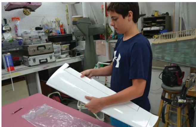
With the exception of the elevator, all of the flight surface hinges are pre-installed. Here Chris (above left) makes sure the flaps are secure. Because of
