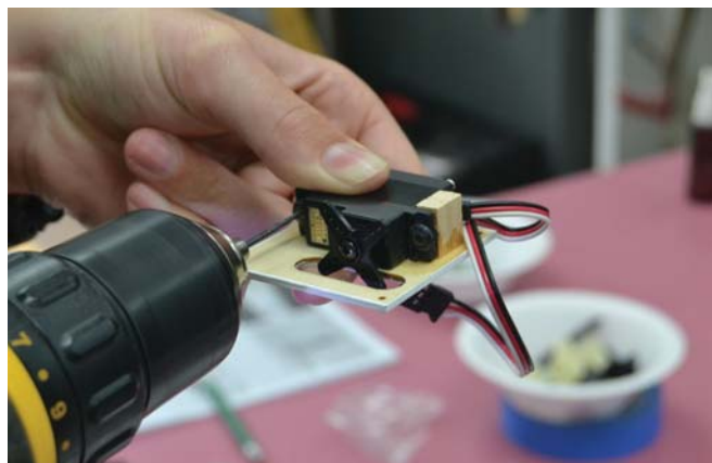
the model's airfoil, micro servos are used on the flaps and aileron surfaces. Futaba S3115 servos (above right) were used in the review model.
