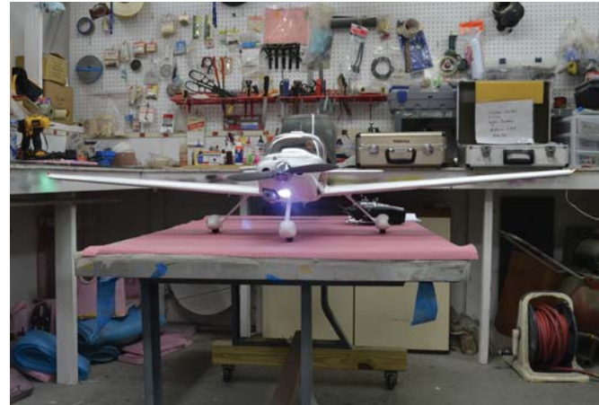
bonus is the addition of the navigation and landing lights. The lights can be set up to turn on independently on a spare channel and are easily seen (above right) in the daytime as well as in the shop.
