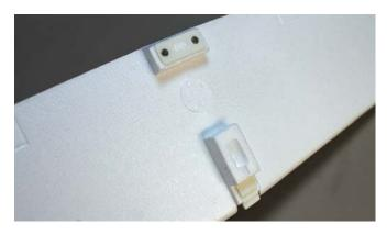
feature in planes of this type. Throw adjustments are handled using U-shaped bends in the pushrods. The tail wheel does not roll, but rather functions as a skid. As do all of the planes in the series, the *Principle* has a pre-mounted cradle (below right) installed the full length of the fuselage to accept the power module. Magnets at the rear of the cradle and tabs and magnets at the front of the cradle keep the module in place, while at the same time allowing it to be easily removed.
