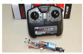
The Tactic SLT receiver built into the power module binds with all Tactic transmitters, including the TTX403 transmitter (above left). Additionally, the receiver can be bound to an AnyLink module fitted to many other transmitter brands. See text for details. The brushless motor is hardwired to a three plug
