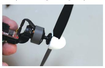
connector on the power module chassis. The prop (above right) connects to the motor by way of a snap-on fitting that allows easy prop changes for each airplane using the module. The fitting also protects the prop, allowing it to pop off rather than break in the event of contact with the ground.
