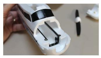
nose pliers to seat the two magnet-tipped pushrods into guide brackets. The wings and the battery hatches are held in place using a combination of magnets and tabs.
