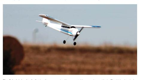
The *Principle* begins its first landing approach with a very stable, nose-down attitude. The high-wing design and flat-bottomed airfoil provide typical trainer-like flight characteristics, even in a model this small.
