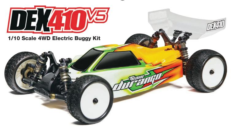
Team Durango engineers have designed the DEX410v5 for more speed, handling and durability than ever. Innovations include a Multi-Axle Driveshaft, an industry first. It lets you "square up" the vehicle's power by changing the driveshaft's length. Use the included medium-length 60 mm driveshaft, or select a short 57.5 mm or long 62.5 mm driveshaft (sold separately) to customize further. With its vast array of highend upgrades, the DEX410v5 is sure to take you to the winner's circle!
