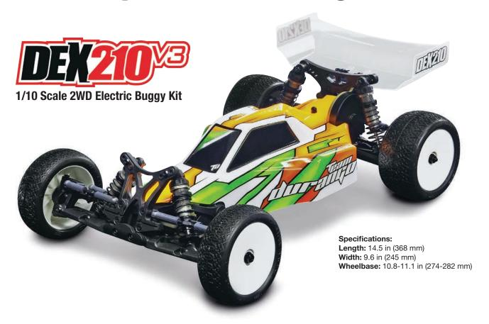
The upgrades to the DEX210v3 are subtle, but out on the track they change the game in a big way. The supreme adjustability of the Multi-Axle Driveshaft and multiple motor positions pays off when you blow through track conditions that have other drivers crashing. The patent-pending Multi-Axle Driveshaft allows for different length driveshaftshelping you get a grip on the track, and the winner's trophy!
