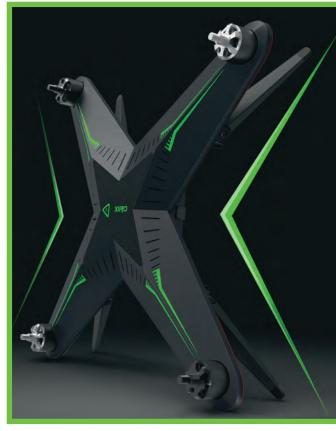
With a shared diagonal of 350 mm (approximately 13.75 inches), Xplorers are among the largest in the company's growing drone selection. Three models—the Xplorer, Xplorer G with a GoPro-compatible 3-axis gimbal and the Xplorer V with a 3-axis gimbal and a digital camera—offer pilots of all types an Xplorer just right for their needs. And if needs change, the Xplorer can be upgraded to the G or V version with already available options.
