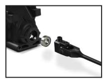
Premium aluminum inserts reduce friction wear and heat. All are factory-molded into the gearbox cases for added security.
