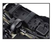
Multiple battery layout options allow racers to create custom weight configurations for faster lap times and improved agility.
