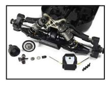
The innovative front/rear gearbox and differentials provide hassle-free servicing and faster tuning options.
