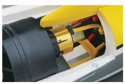
The fuselage section over the shroud and motor can be removed easily with gentle finger pressure, but holds tight in flight, even at top speed.
