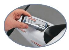
A hatch in the top of the plane provides easy access to the battery.
