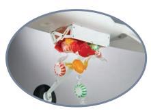
Operate the "drop-door" from the 5th channel of the radio for in-flight deployment of a parachute or other creative payloads!
