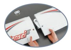
The wing halves slide together onto a tube and secured with two bolts.
