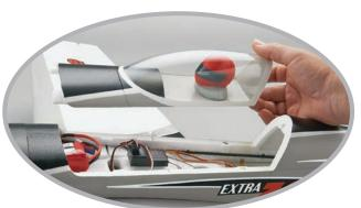
The hatch is held securely in place with magnets, which allow for quick LiPo replacement and access to the plane's on-board gear.
