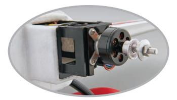
The 30-35-1000kV brushless motor provides plenty of power for executing extreme 3D maneuvers.
