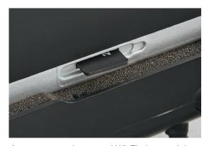
A memory card port and Wi-Fi give modelers the option to store videos and photos onboard, or stream directly to the web.
