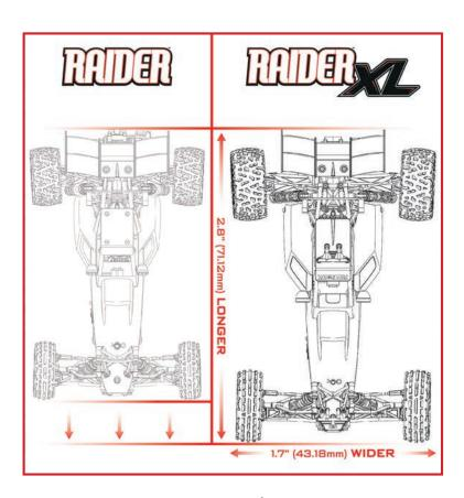
With its longer wheelbase and wider stance, the RAIDER XL is 20% larger than the 1/10 scale RAIDER.
