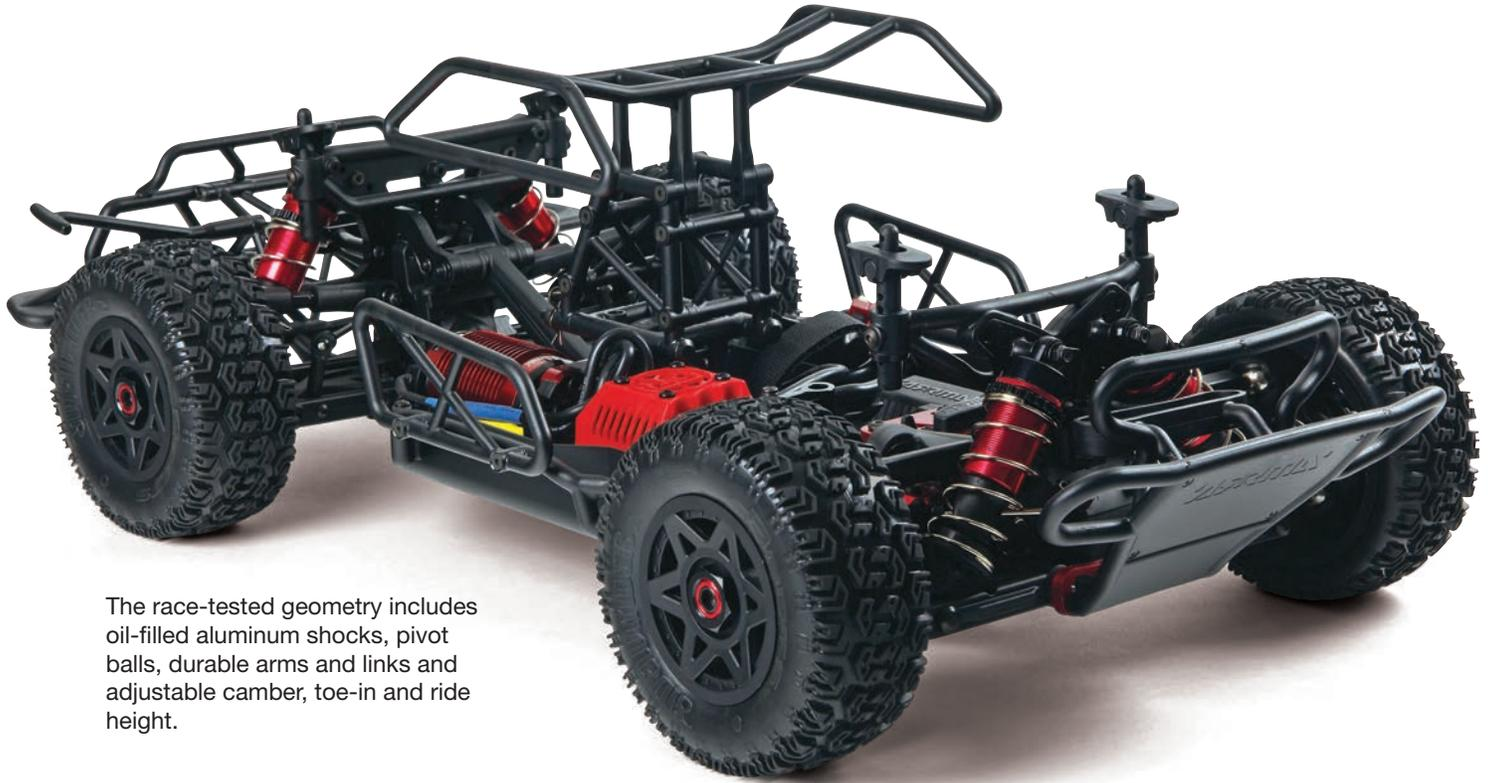
The race-tested geometry includes oil-filled aluminum shocks, pivot balls, durable arms and links and adjustable camber, toe-in and ride height.
