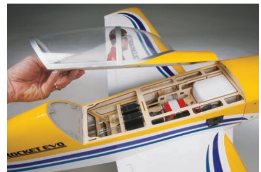
The large battery compartment allows for easy access to onboard components.
