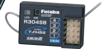
The 4PLS includes an R304SB 2.4GHz receiver.
