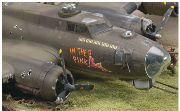
In that most B-17's taxied on their outboard engines, only the bottom blade of the inboard prop was bent, whereas the whirling blades of the outboard propeller were severely distorted by the mishap. The blades are bent as described in the text. Note the nose art on this B-17. Though you may wish to copy an actual aircraft, you can also create your own nose art, as our modeler did.
